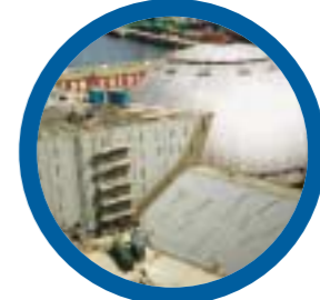
Free-standing Moss ship under construction at Hyundai Heavy Industries, South Korea
